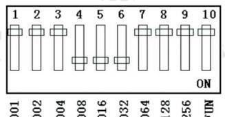
If you want to set the 6 addresses of the decoder 57, 58, 59,60,61,62, and the you should set the beginning address 57, so the 4th, 5th, 6th in down position ON, other position OFF 4th = 008.5th = 016.6th = 032
